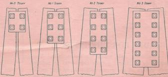
used to secure the needed strength plus a liberal margin of safety. Tower plates with six bolt holes are used on towers designed for 8-foot mills. A set of these plates with 24 bolts securely tightened makes a tower much stronger and more rigid at the top than bands of short girts near the top. Illustrations above show the tower plates used on No. 0, 1, 2, and 3 towers.
